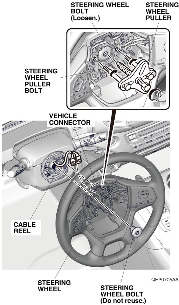
9. Using a steering wheel puller, release the steering wheel. Do not thread the steering wheel puller bolts in more than 5 mm (0.20 in.). When removing the steering wheel, take care not to move the front wheels.
