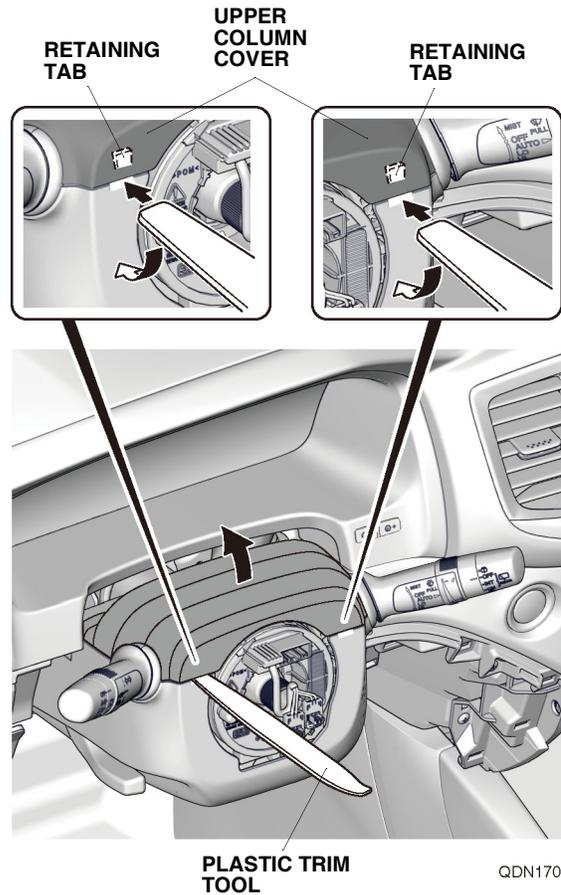
13. Release the upper column cover, and secure it to the dashboard with masking tape.
