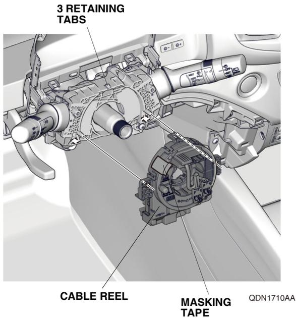
18. Remove the masking tape. Remove the steering angle sensor.
