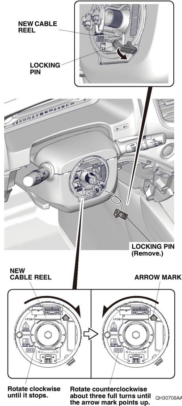
37. Before installing the new steering wheel, make sure the front wheels are still pointing straight-ahead. To confirm the cable reel is line up properly, rotate the cable reel clockwise until it stops, then rotate it counterclockwise about three full turns. The arrow mark on the new cable reel label must point straight up.
