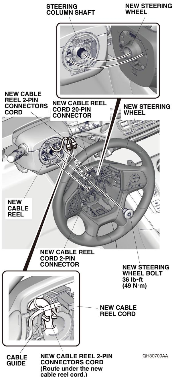
39. Install the new steering wheel bolt. Torque the new steering wheel bolt to 36 lb-ft (49 N·m). Tighten at the specified torque within 5 minutes.
