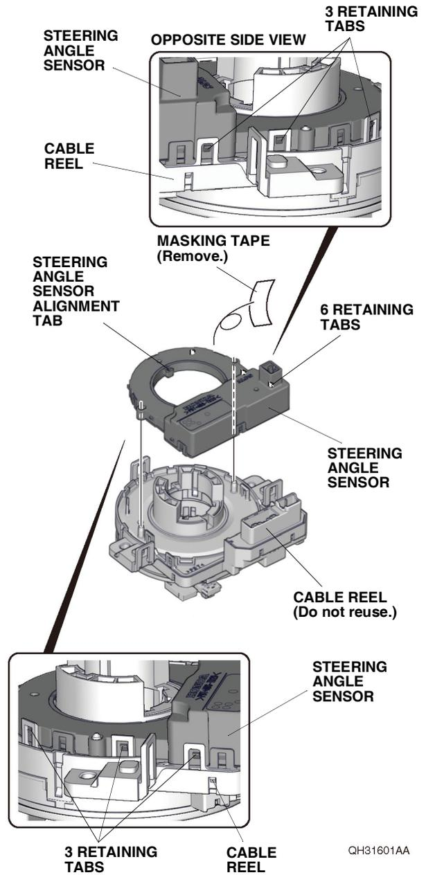
19. Install the steering angle sensor to the new cable reel with six retaining tabs.
