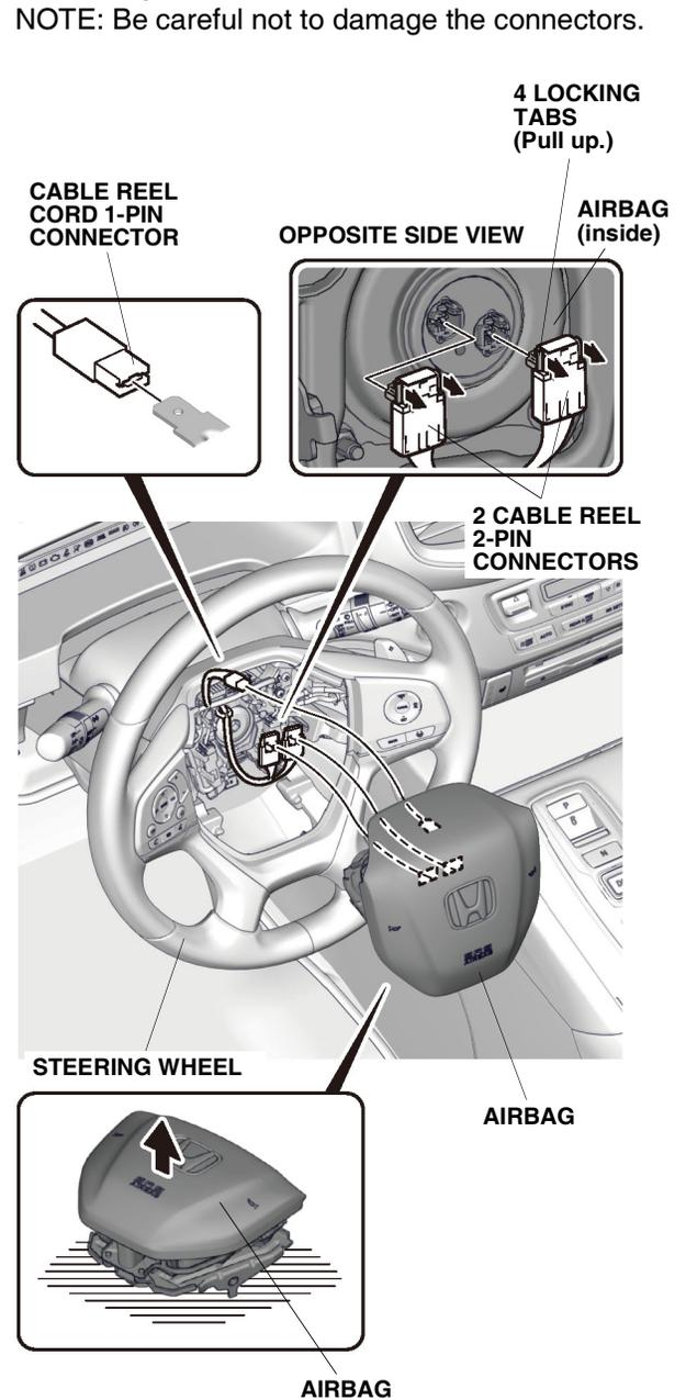
7. Remove the airbag. Do not drop the removed airbag or hit it on an object. Place the removed airbag in a safe place with the padded surface (top) facing up.
