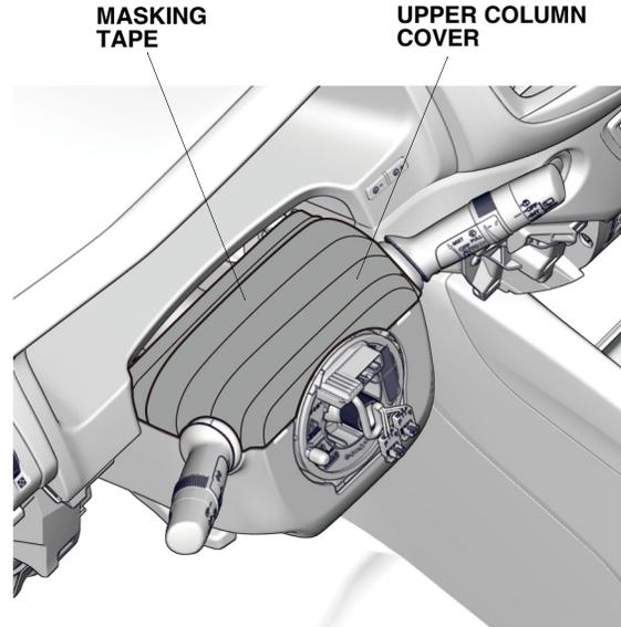
12. Using a plastic trim tool, release the two retaining tabs.
