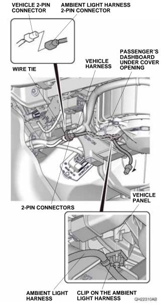
11. Route the ambient light harness as shown, and secure it to the vehicle panel with the clip on the ambient light harness.
