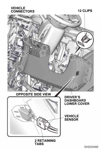
5. Remove the tape to free the vehicle 2-pin connector.
