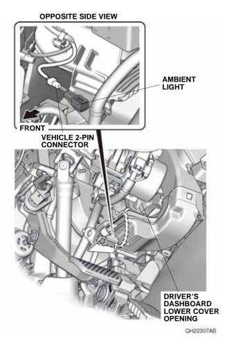
Install the ambient light to the passenger's dashboard under cover as shown.
