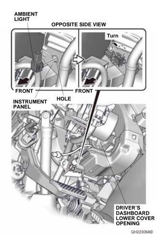
7. Plug the vehicle 2-pin connector into the ambient light.
