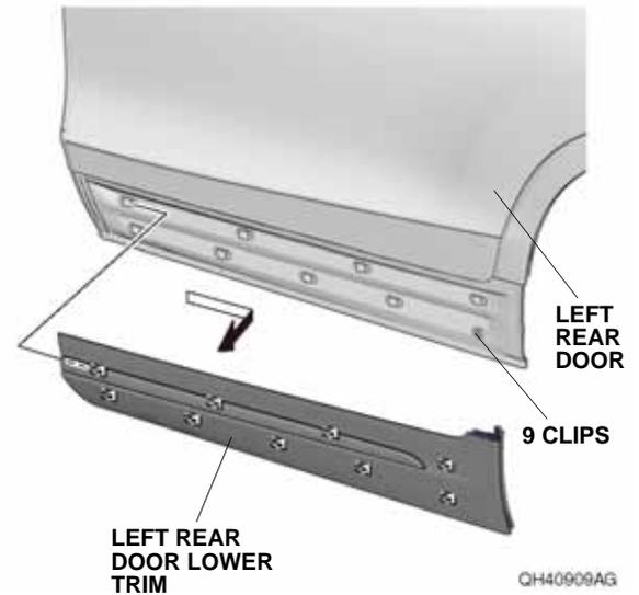
9. Remove the nine clips from the left rear door as shown.
