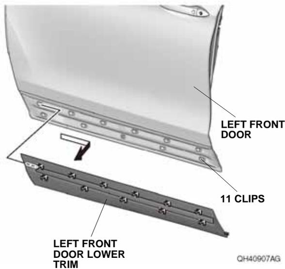
3. Remove the eleven clips from the door as shown.
