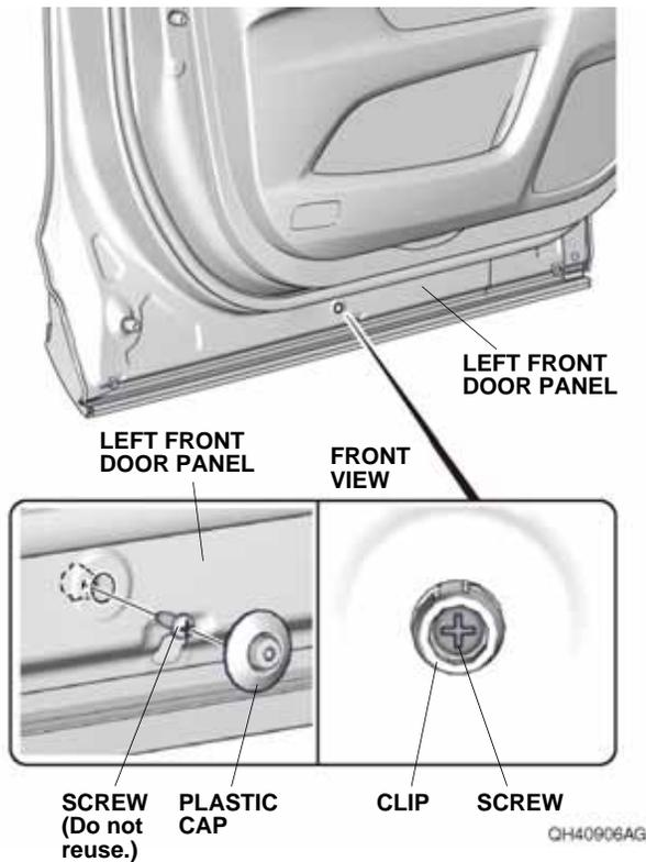
2. Slide the left front door lower trim back and out to remove it.
