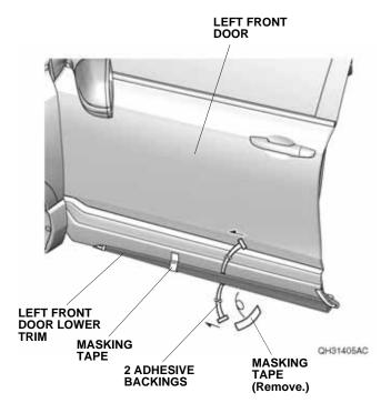
Using the rubber roller, apply firm pressure against the center of the left front door lower trim. Start from the rear side, and roll the left front door lower trim as shown. Apply firm pressure for 30 seconds at 100 mm (3.94 in.) increments.
