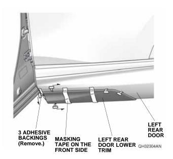
19. Using the rubber roller, apply firm pressure against the front of the left rear door lower trim. Start from the front side, and roll the left rear door lower trim as shown. Apply firm pressure for 30 seconds at 100 mm (3.94 in.) increments.
