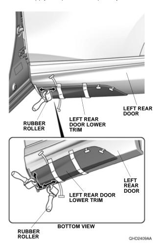
20. Remove the masking tape. While applying light pressure against the left rear door lower trim, carefully remove the adhesive backings up to the edge of the remaining masking tape.
