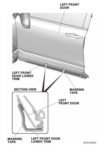
6. While applying light pressure against the left front door lower trim, carefully remove the three adhesive backings as shown.
