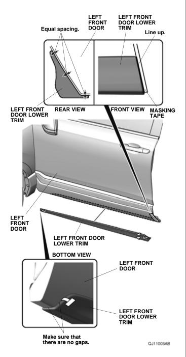
5. Loosely secure the left front door lower trim to the left front door with masking tape as shown.
