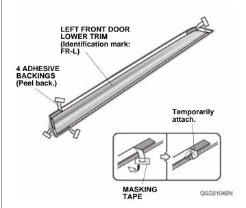
4. Line up the left front door lower trim with masking tape as shown.
