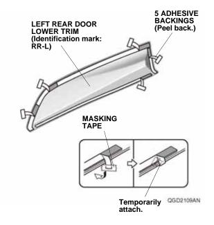
16. Line up the left rear door lower trim as shown. NOTE: Make sure that there are no gaps between the left rear door and the left rear door lower trim.
