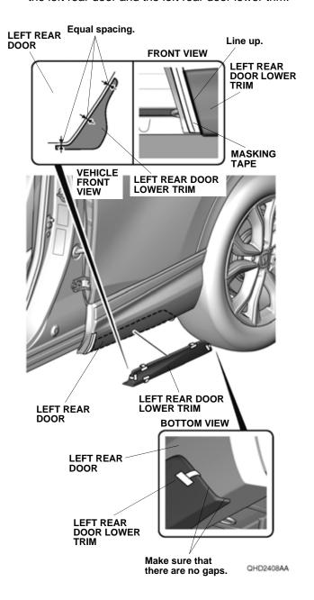
17. Open the left rear door. Loosely secure the left rear door lower trim to the left rear door as shown.
