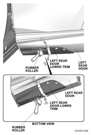
22. Remove the masking tape. While applying light pressure against the left rear door lower trim, carefully remove the adhesive backings as shown.
