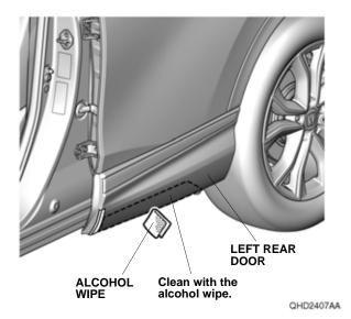
15. Peel back the adhesive backings, and tape them to the front surface of the left rear door lower trim with masking tape.
