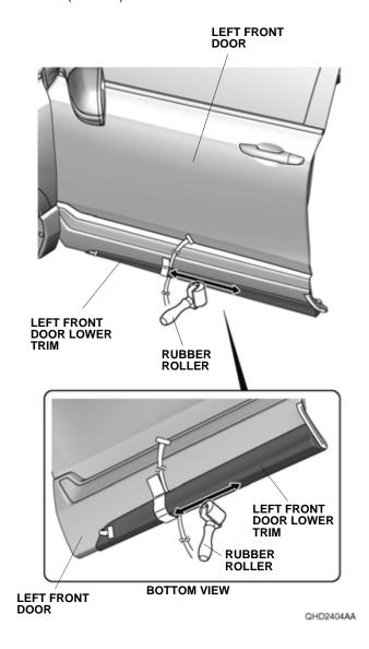
10. Remove the masking tape. While applying light pressure against the left front door lower trim, carefully remove the adhesive backings as shown.
