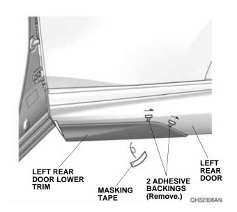
23. Using the rubber roller, apply firm pressure against the rear of the left rear door lower trim. Start from the front side, and roll the left rear door lower trim as shown. Remove the masking tape.
