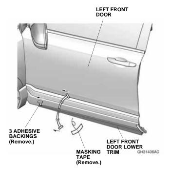
11. Using the rubber roller, apply firm pressure against the front of the left front door lower trim. Start from the rear side, and roll the left front door lower trim as shown. Remove the masking tape.
