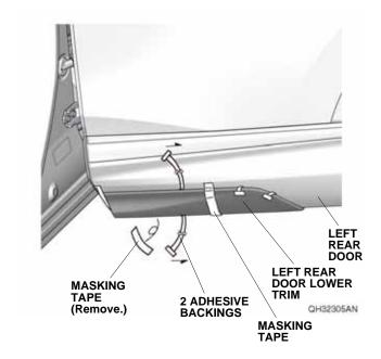
21. Using the rubber roller, apply firm pressure against the center of the left rear door lower trim. Start from the front side, and roll the left rear door lower trim as shown. Apply firm pressure for 30 seconds at 100 mm (3.94 in.) increments.
