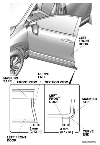
Using the alcohol wipe, thoroughly clean the left front door where the left front door lower trim will attach.
