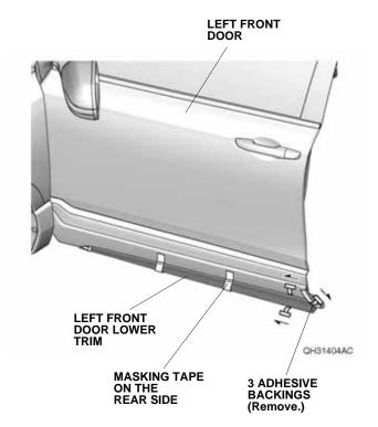
7. Using the rubber roller, apply firm pressure against the rear of the left front door lower trim. Start from the rear side, and roll the left front door lower trim as shown. Apply firm pressure for 30 seconds at 100 mm (3.94 in.) increments.
