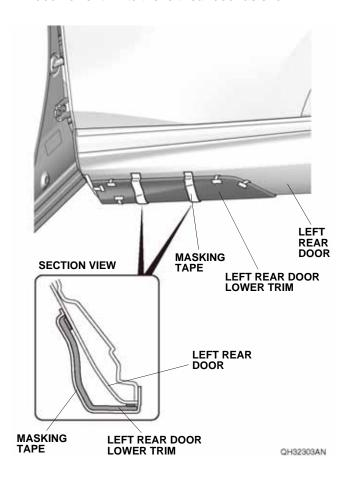
18. While applying light pressure against the left rear door lower trim, carefully remove the taped adhesive backings up to the edge of the masking tape on the front side as shown.
