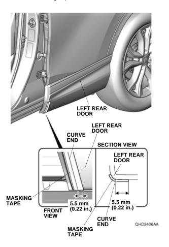
14. Using the alcohol wipe, thoroughly clean the left rear door where the left rear door lower trim will attach.
