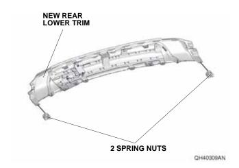
17. Install the new rear lower trim to the rear bumper with 10 retaining tabs, and two bolts removed in step 8. Then, plug the vehicle connector, and secure the vehicle clip to the Hands-Free Access unit (if equipped).
