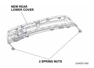
Install the new rear lower cover to the new rear lower trim with six retaining tabs, two clips, and two bolts removed in step 10.
