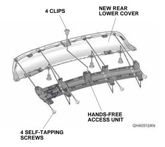
14. Install the two spring nuts removed in step 11 to the new rear lower cover.
