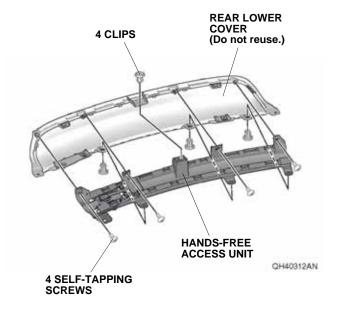
13. Install the Hands-Free Access unit to the new rear lower cover with four clips and four self-tapping screws removed in step 12.
