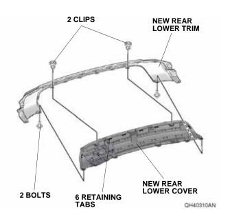
Install the two spring nuts removed in step 9 to the new rear lower trim.
