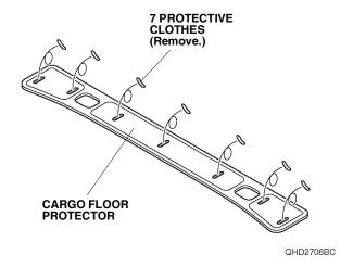
Position the cargo floor protector on the cargo floor. Line up the cargo floor protector with the tie-down hooks on the cargo floor as shown. Secure the cargo floor protector to the cargo floor with seven fasteners.
