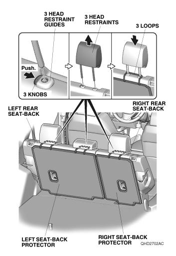
3. Fold down the left and right rear seat-backs, and peel back the left and right cargo floor lids. Line up the left and right seat-back protectors with the tether anchor covers on the left and right rear seat-backs as shown. Secure the left and right seat-back protectors to the left and right rear seat-backs with 15 fasteners.
