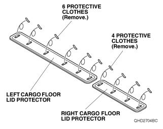
5. Position the left and right cargo floor lid protectors on the left and right cargo floor lids as shown. Secure the left and right cargo floor lid protectors to the left
