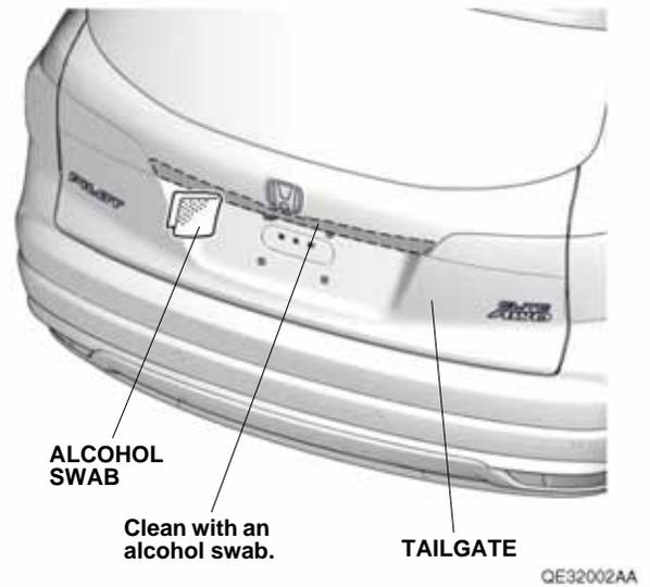
2. Peel back the adhesive backings, and tape them to the front surface of the tailgate chrome trim with masking tape. Remove the small piece of adhesive backings.
