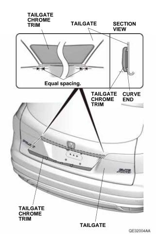
4. While applying light pressure against the tailgate chrome trim, carefully remove the taped adhesive backings.
